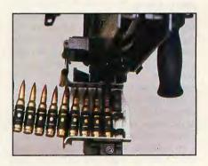
SS-77 stainless steel feed tray. Note slots on the tray which help to retain the R1M1 links. Photo: courtesy Lyttelton Engineering Works
